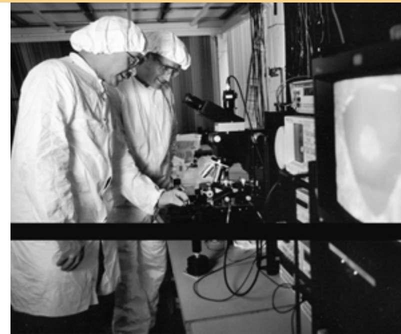
Using a high-powered microscope hooked up to a VCR, Dorian Liepmann (rear) and Al Pisano, in clean suits and safety glasses, examine the silicon carbide micro-rotor on the monitor, checking for manufacturing tolerances and changes they could make to refine the rotor’s fabrication.
