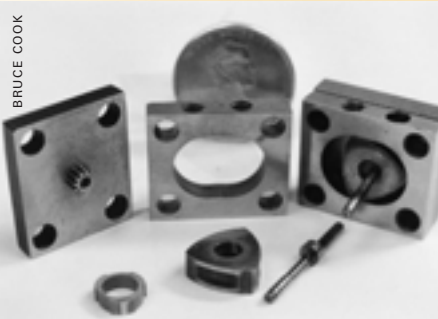
Detail of the penny-sized MEMS mini-engine. On the right, the mini-engine is assembled; center and left, it is pulled apart showing the triangular rotor (center foreground), output shaft, gear, and housings.
