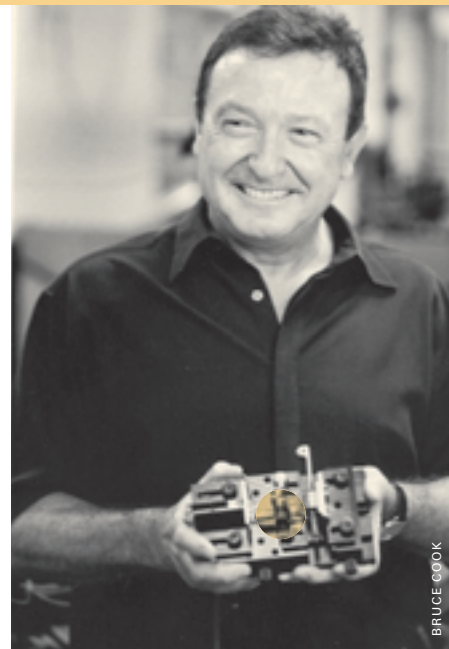
"We're in the business of shrinking," says Carlos Fernandez-Pello, holding a working model of the mini-combustion engine test bench. Shown here is not only the penny-sized engine (see highlight), but all the peripheral equipment from small-scale clutches and ignition systems to a dynamometer for measuring power output. The mini-engine runs partially under its own power.
